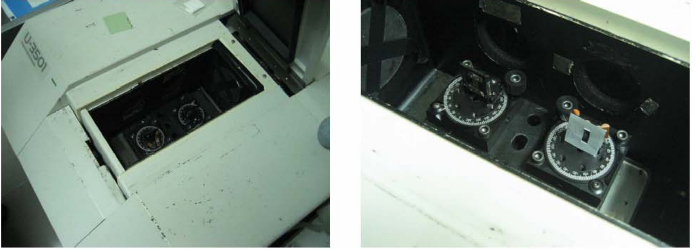
Figure 1: The overview of Hitachi U-3501 spectrometer (left), and the sample holder in the spectrometer (right).
