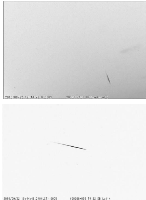
Fig. 2 Two Meteor Cameras being operated 200 km apart captured the same meteor.
