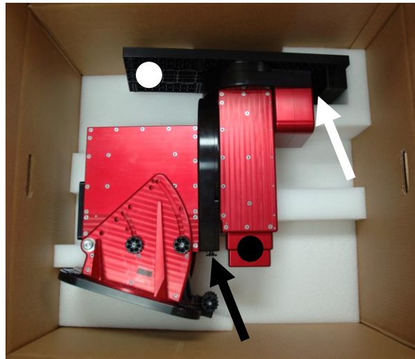
Figure 1: The black arrow points to the right ascension balance knob; the black circle indicates where to grasp and wiggle the right ascension axis during engagement. The white arrow points to the declination balance knob; the white circle indicates where to grasp and wiggle the declination axis during engagement.
