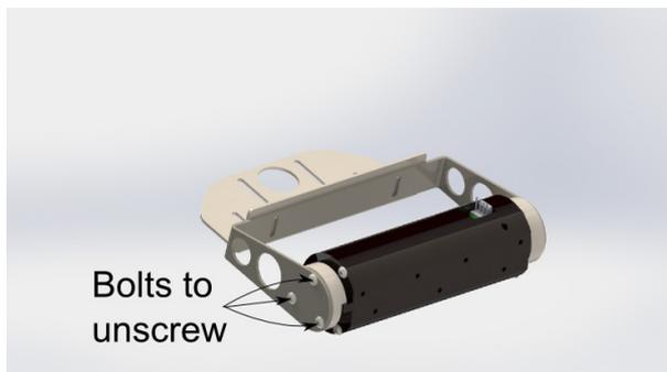
*Fig. 4: The last bolts that need to be unscrewed are the ones in the drive wheel*
