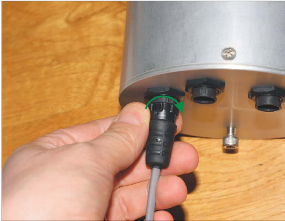
Fig. 5 Then turn the connector's collar in clockwise fashion
