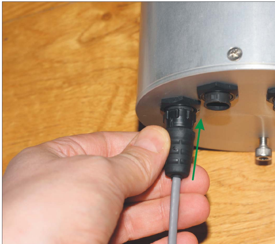
Fig. 4 Push the connector straight
