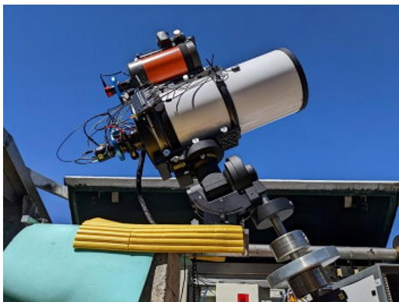
Figure 1. Robotic Lulin Lunar Impact Flashes Telescope was installed at one of the TAOS Domes.
