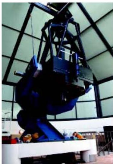
Lulin One-meter/Optical Telescope
