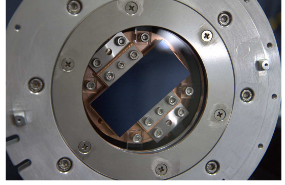
Figure 11: The engineering grade CCD chip installed in the dewar. The chip is supported by the copper plate. The window in front of the CCD is fused silica.
