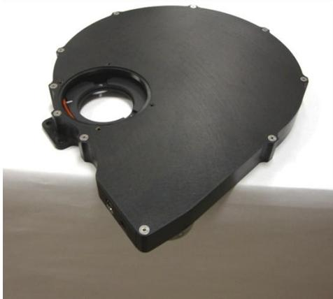
Remove the lid, making sure not to damage the light guard sticker of the connector face. Set aside the lid and ten flathead screws for now. Take a moment to inspect for any packing materials or dust inside the wheel, remove using compressed air or wipe.
