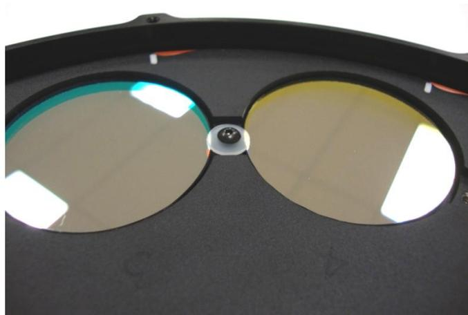
Install filters using the below screws and nylon washers provided using the 1/16" Allen wrench provided. **DO NOT OVER TIGHTEN**; this may physically distort your filters which will optically distort your image. Make sure filters do not move after tightening. Rotate the carousel by hand to verify clearance under the circuit board.
