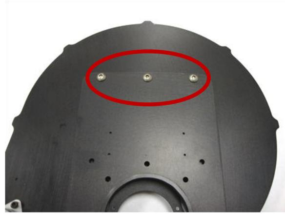
Flip Filter Wheel right side up and set on the edge of a table. The motor should hang off the side so the housing does not rock back and forth. Remove the ten #6-32 x 5/16 flathead screws from the perimeter of the lid using the 5/64 Alan wrench provided.
